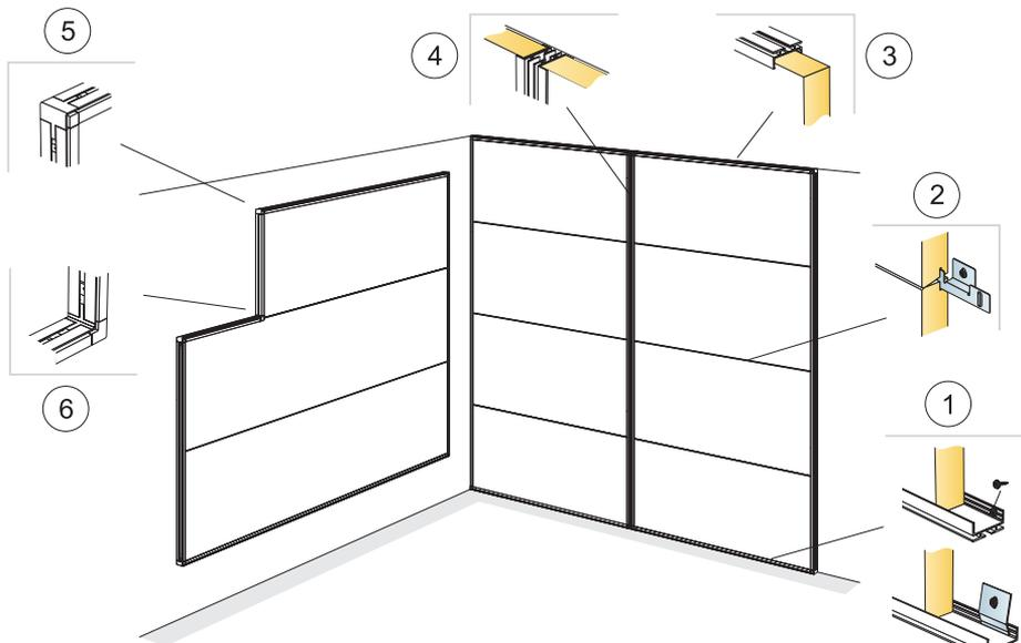
1. Connect WP Profile L=2687 mm, fixed (alt. with Connect Fixing bracket 0214) at 400 mm centres.
