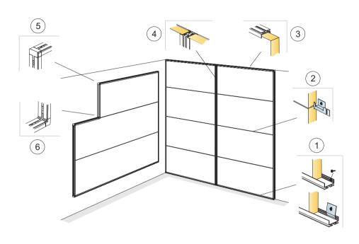
1. Connect WP Profile L=2687 mm, fixed (alt. with Connect Fixing bracket 0214) at 400 mm centres.
