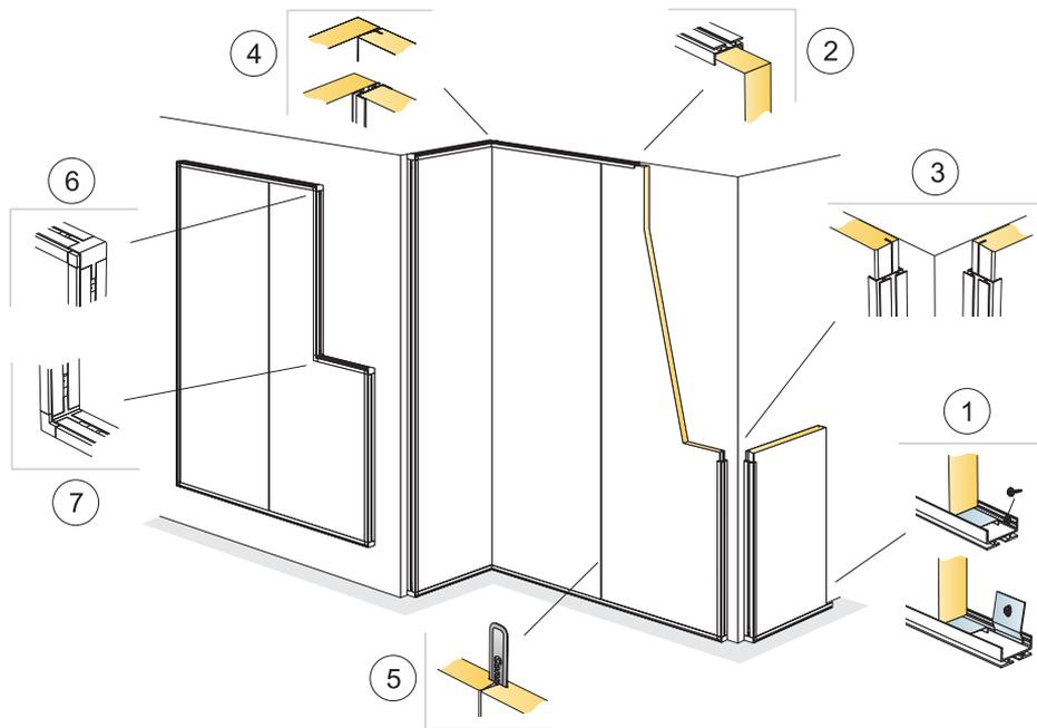
1. Connect WP Profile L=2687 mm, fixed (alt. with Connect Fixing bracket 0214) at 400 mm centres, with Connect WP Space bar, L=2400 mm.
