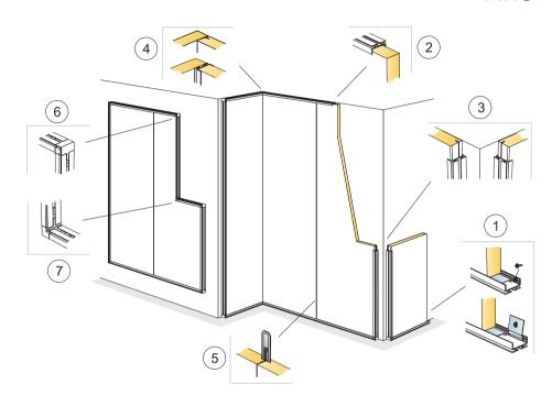
1. Connect WP Profile L=2687 mm, fixed (alt. with Connect Fixing bracket 0214) at 400 mm centres, with Connect WP Space bar, L=2400 mm.
