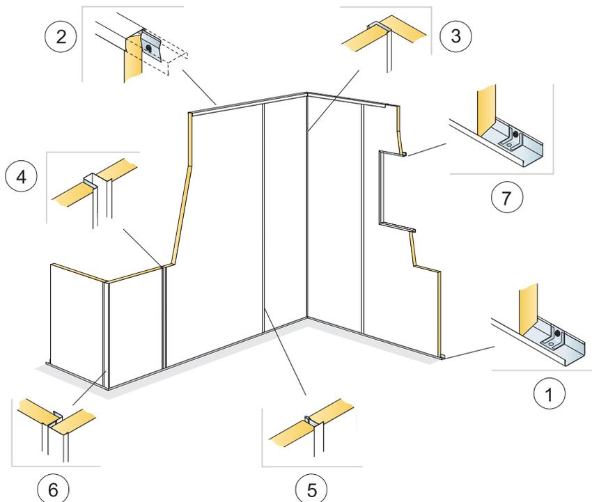
1. Connect Channel trim 0465, L=2700 mm, fixed at 300 mm centres. Connect Direct fixing plate 0032 is placed inside at each fixing point if Wall Panel is not supported by the floor.
