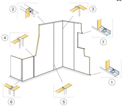
1. Connect Channel trim 0465, L=2700 mm, fixed at 300 mm centres. Connect Direct fixing plate 0032 is placed inside at each fixing point if Wall Panel is not supported by the floor.
